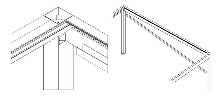
Check that all the "U" profile holes match the M6 pre-drilled ones on the beam. If all of them match, apply the sealant between the "U" profile and the beam after screwing the profiles with the ULS (ISO 7380) A2x16 screws.
