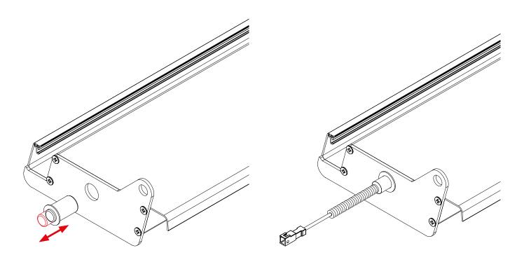
The slats with LED come already pre-instaled on one side with a hollow axle. The LED connector comes through this axle and it has a protection spring. The O-210 retractable axle needs to be installed on the other end.
