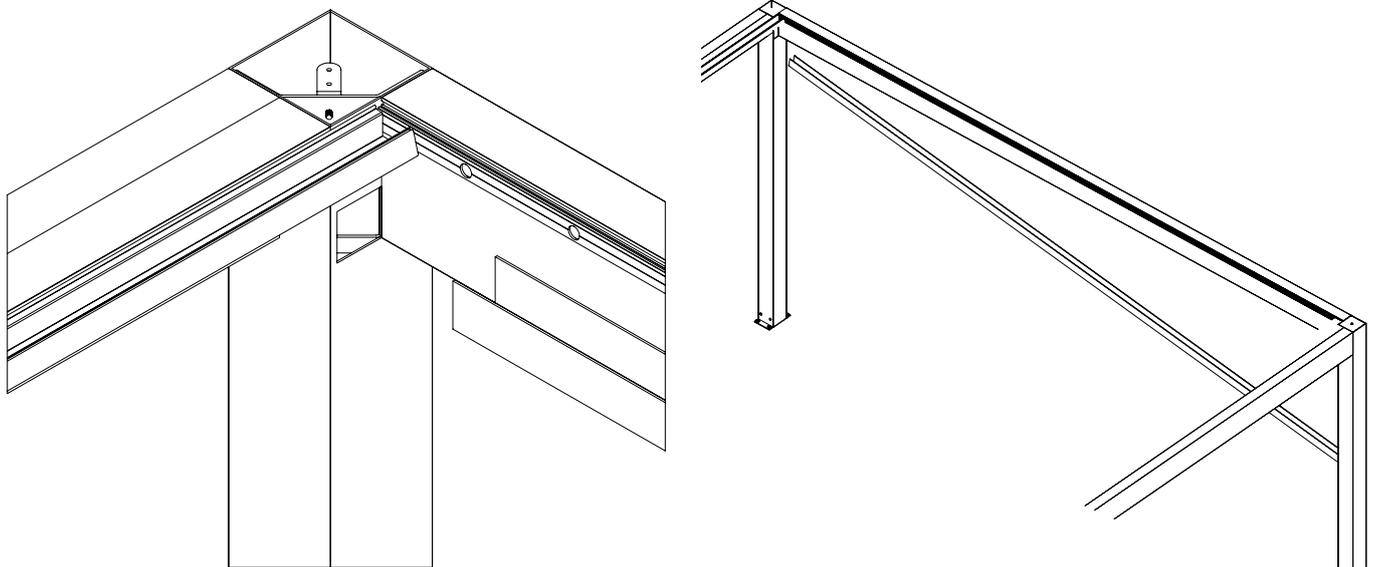
Check that all the "U" profile holes match the M6 pre-drilled ones on the beam. If all of them match, apply the sealant between the "U" profile and the beam after screwing the profiles with the ULS (ISO 7380) A2x16 screws.
