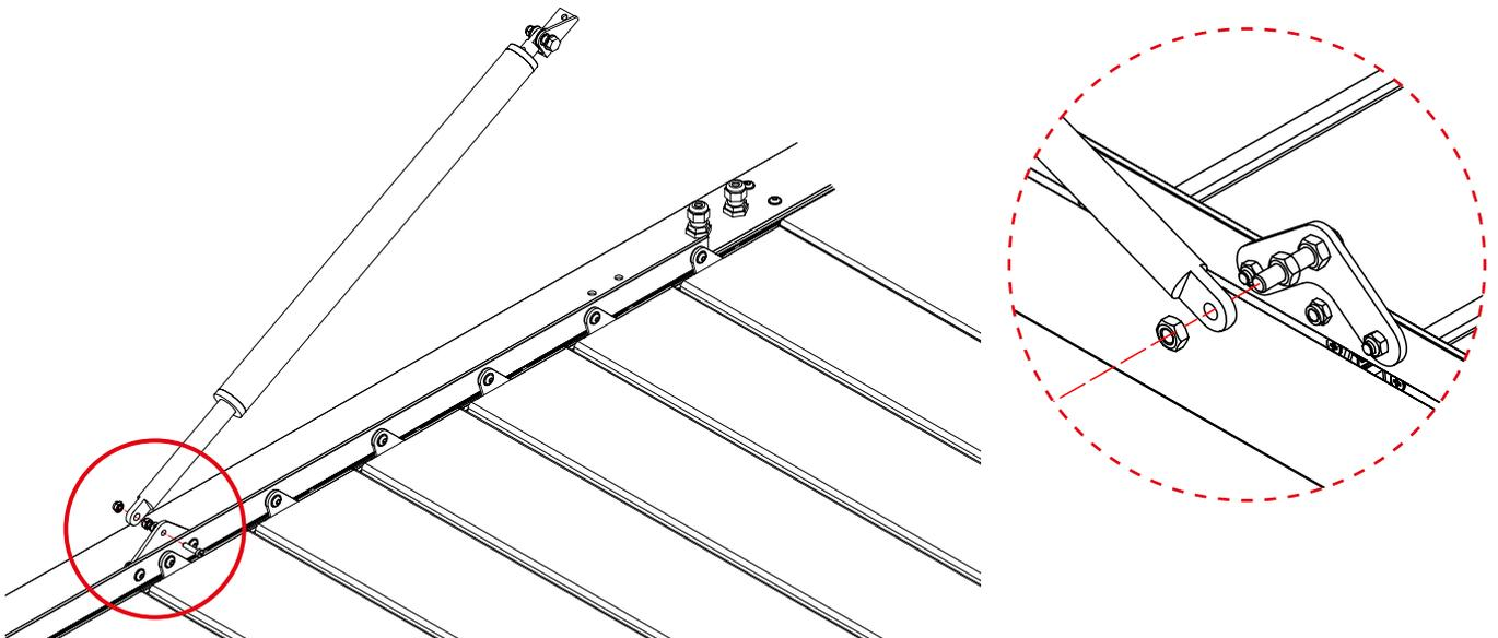
3 Move the motor opening the pergola until the bracket can be screwed onto the threaded holes of the beam.
