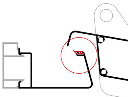
Installing rubber on the slats (150 to 160 slat step).
