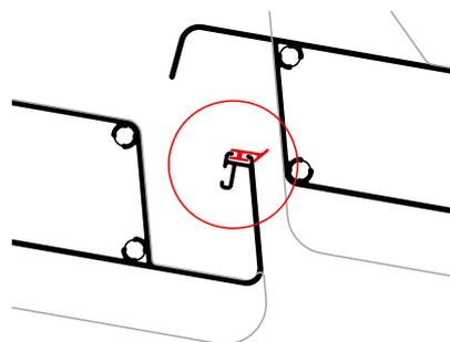
Installing rubber on the slats (150 slat step).
