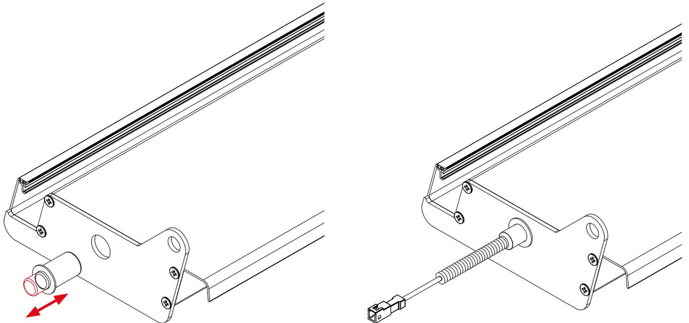
The slats with LED come already pre-installed on one side with a hollow axle. The LED connector comes through this axle and it has a protection spring. The O-210 retractable axle needs to be installed on the other end.
