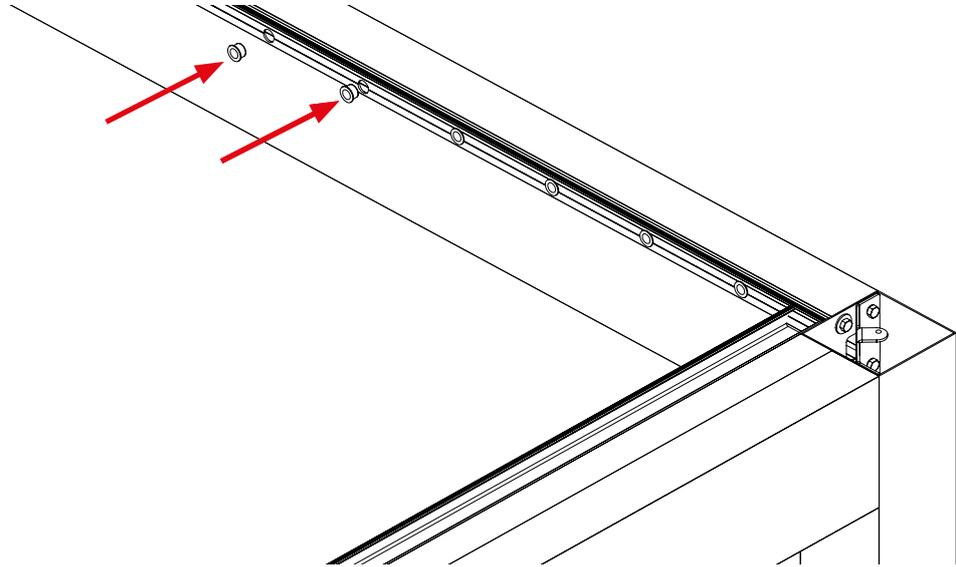
To install the slats without LED you will have a set of O-210 pivot-type caps, integrated by a 16,4x25 mm plastic cap and a retractable stainless steel axle.
