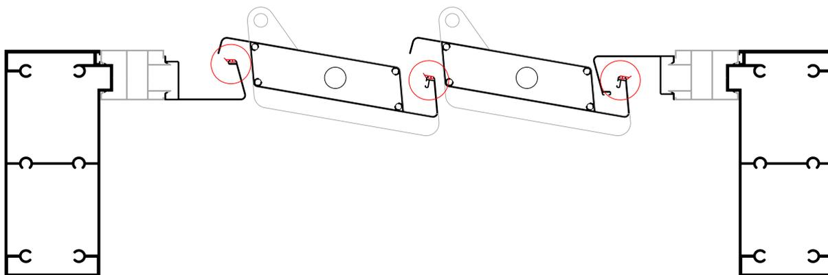
Installing rubber on the clippable opening gutter.
