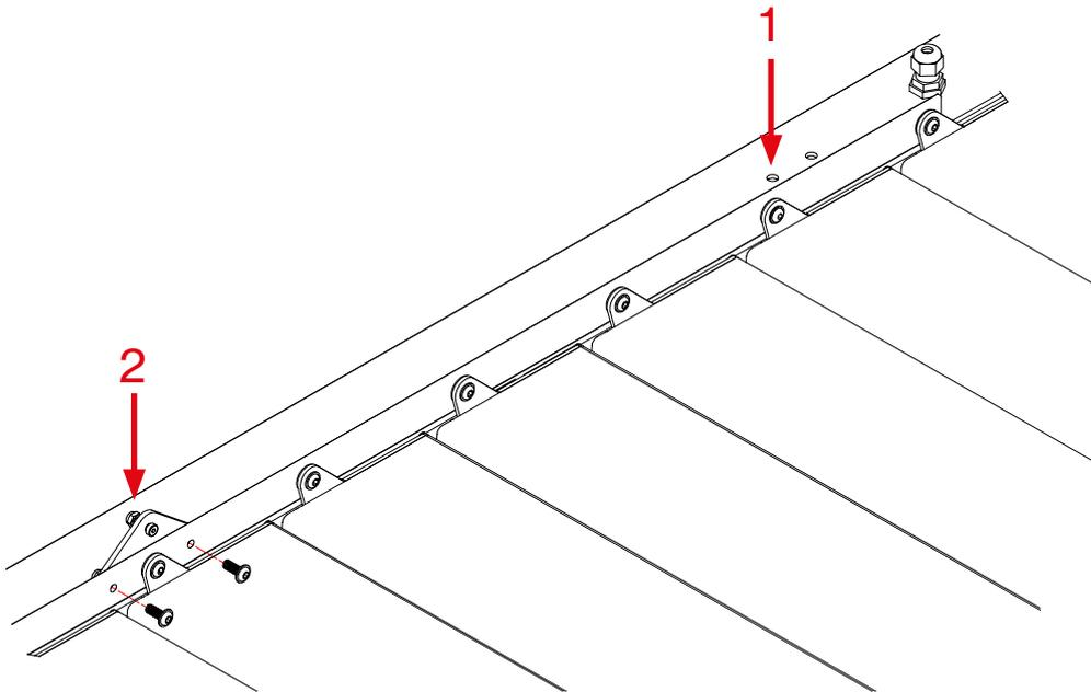
Steps to join the motor to the transmission plate.
