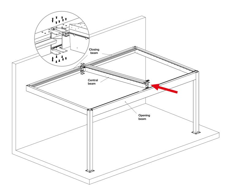
With the **central** beam in place, proceed to fix it as shown in the image.
