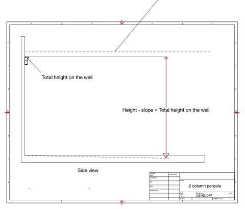
ATTENTION: Leave a clearance of 100 mm above the beam for the slats to turn.
