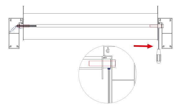
Using a No 4 Allen key, pull back the axle until it stops in the grooved hole.
