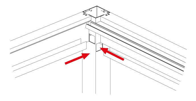
Check that all the "U" profile holes match the M6 machined ones on the beam. If all of them match, apply the sealant between the "U" profile and the beam after screwing the profiles with the ULS (ISO 7380) A2 M6x16.
