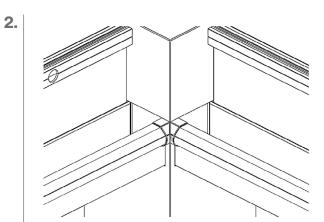
Fit the perimeter LED corner piece shown in the picture on the right to the **corners of the pergola with a mitre**.
