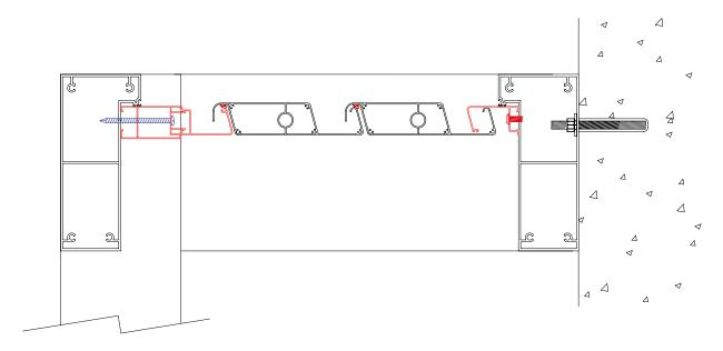
Check that all the "U" profile holes match the M6 machined ones on the beam. If all of them match, apply the sealant between the "U" profile and the beam after screwing the profiles with the ULS (ISO 7380) A2 M6x16.
