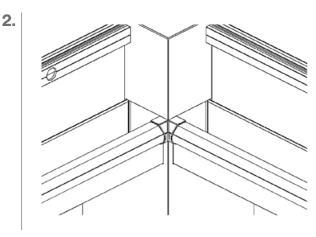
Fit the perimeter LED corner piece shown in the picture on the right to the corners of the pergola with a mitre.
