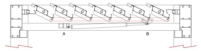
4. Finally we reinstall the motor support in the "U" profile with its 2 screws (A).
