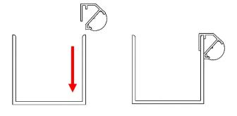
Fit the perimeter LED corner piece shown in the picture on the right to the **corners of the pergola with a column**.
