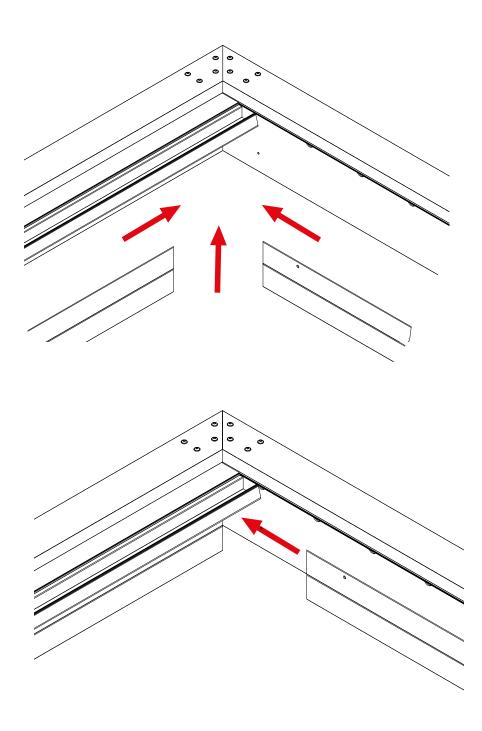
Check that all the "U" profile holes match the M6 machined ones on the beam. If all match, apply sealant between the U-profile and the beam and around the screw holes, then screw the profiles together using ULS (ISO 7380) A2 M6x16 screws.
