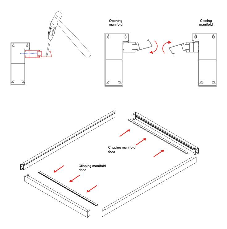
Apply sealant supplied between the mating faces of the clip-on siding on the **opening** and **closing** beam and respective manifolds. We then clip the opening and closing manifolds. We will possibly need to use clamps or wooden blocks to help with the clipping.
