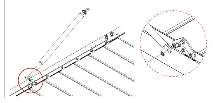
Move the motor opening the pergola until the bracket can be screwed on the beam threaded holes. 3.
