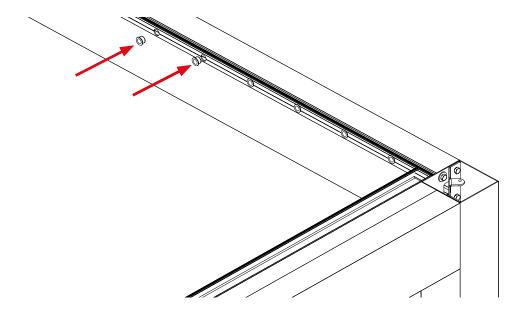
To install the slats without LED you will have a set of O-210 pivot system caps, integrated by a 16,4x25mm plastic cap and a retractable stainless steel axle.
