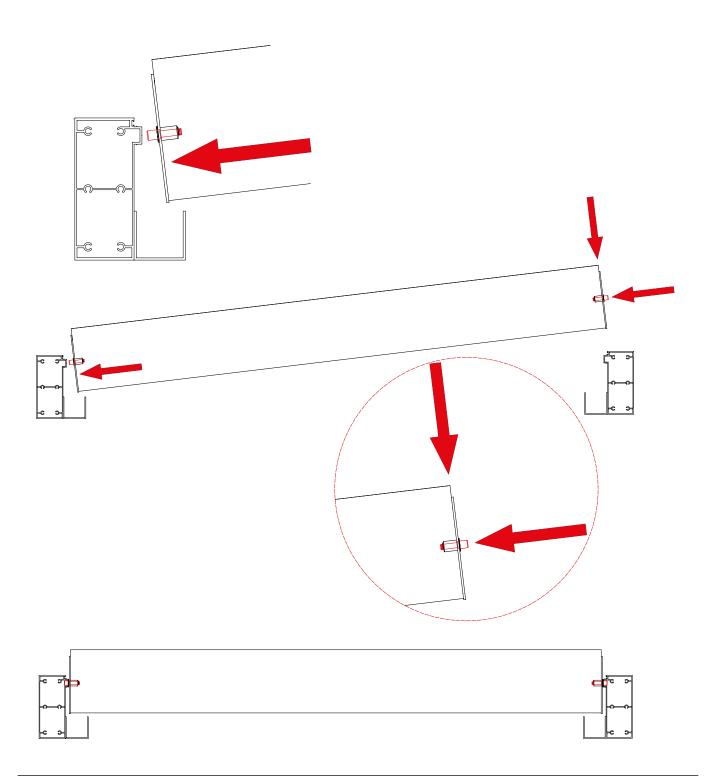
When reaching a hole for LED slats, connect the connector and insert it into the beam (as shown in the images below).
