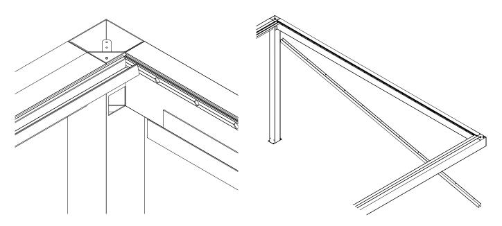
Check that all the "U" profile holes match the M6 machined ones on the beam. If all of them match, apply the sealant between the "U" profile and the beam after screwing the profiles with the USL (ISO 7380) A2x16 screws.
