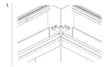
Fit the perimeter LED corner piece shown in the picture on the right to the **corners of the pergola with a mitre**.
