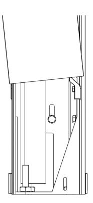
On the left side of the column, clip the profile onto the clipping rubber from the bottom to the top.
