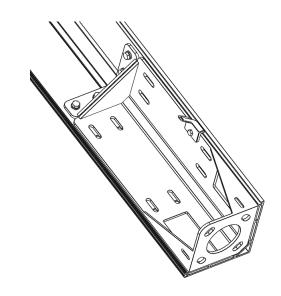
2. Place over the screw DIN 933 A2 M12x50, which will allow the height of the column to be adjusted, and tighten it loosely. (2)
