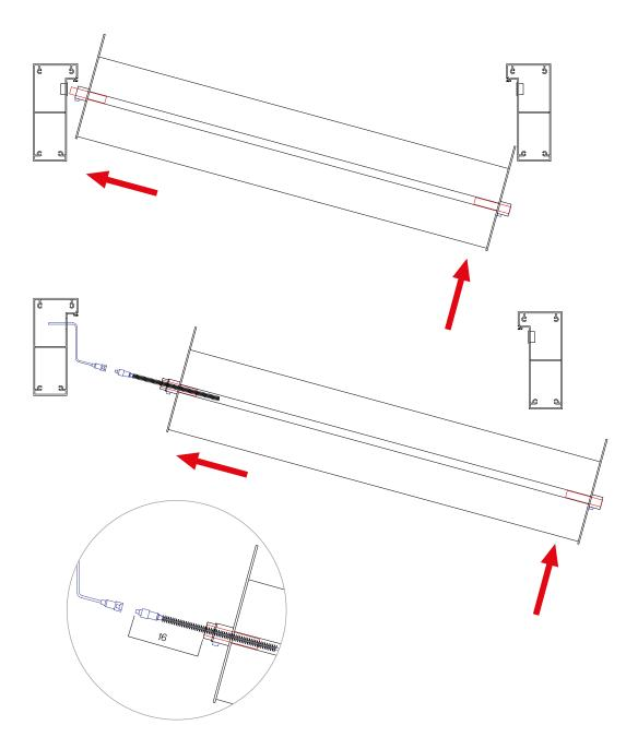
To install the slats, they must be tilted with the end caps facing down, inserting the fixed axle first (left) and then the mobile one (right).
