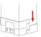
At the end of the assembly after section 7.1 Trim cover. When the height of the column is adjusted, two trim pieces are attached to the base. To fix the trims, they are sealed with silicone.
