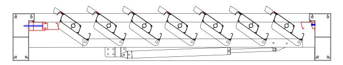
4. Finally we reinstall the motor support in the "U" profile with its 2 screws (A).
