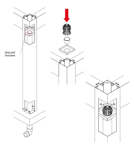
Finally, apply the sealant (included) all around the perimeter of the collecting tray and the adapter, as shown in the picture (sealant in red), and insert the universal leaf guard into the adapter.
