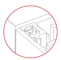
Slightly unscrew the screw on the upper part of the right-hand clipping piece of the trim profile in order to be able to put the profile in place. Then tighten the screws again until the column is completely closed.
