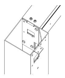
Screw two ULS ISO 7380 M6x16 screws into the column fitting at the top of the beam before fitting the other screws
