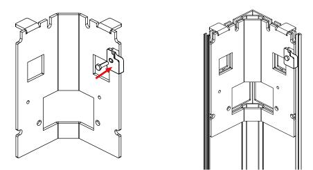
Check that the closing beam is level to the base, its height from the plan and that all markings form a 90° angle with the base brackets. The correct installation of the beam and the bases is critical for the optimum operation of the pergola.
