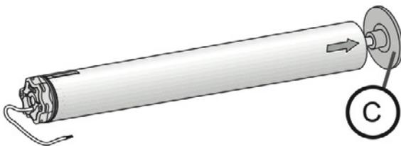
**2.4.1** Assemble the tube-motor set on the end support (C).
