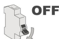
**a)** Cut the electrical power to the awning before performing any maintenance procedures.
