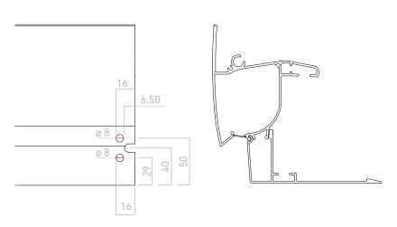
Cutout for the motor cable passage and hole for the limit switch adjustment.
