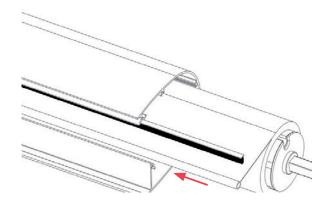
Push the shaft, with the canvas and bushes, into the box profile. Also insert the mat into the box profile, cutting off the excess brush.
