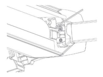
Adjust the height of the elbow so that it closes the box perfectly (if you are using a machine, before adjusting it hold the arms with their cover and release the canvas by operating the machine).
