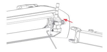
Assemble the Smart arms. Mount the arms in their housing, insert the solid shafts and fix them with the lower pins. Mount the strips to the front terminals.
