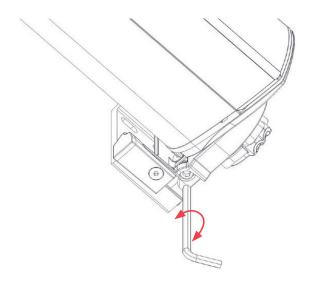
Adjust the inclination of the cassette and then tighten the fixed supports (M6 screws).
