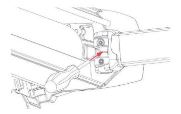
Detail of the extraction of the shaft in cases where disassembly is required.
