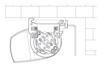
When mounting, leave enough wall clearance for the adjustment key.
