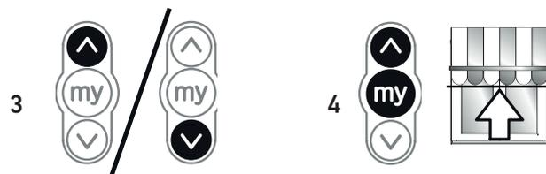
3. If necessary, adjust the position of the awning using the raising and lowering buttons.
