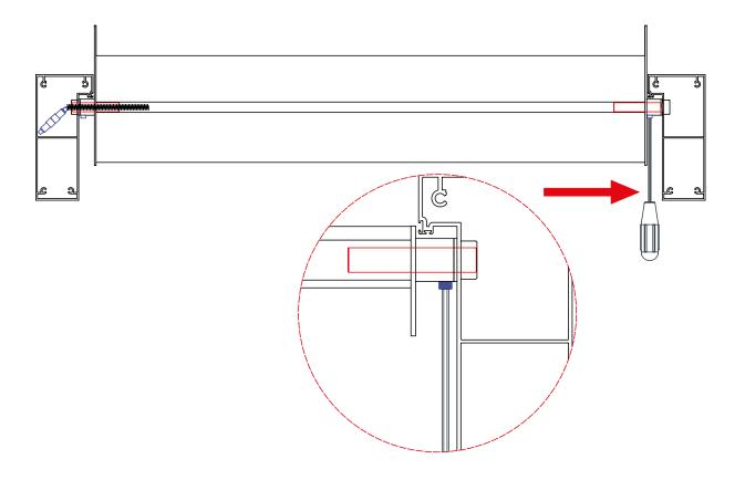
Using a No 4 Allen key, pull back the axle until it stops in the grooved hole.
