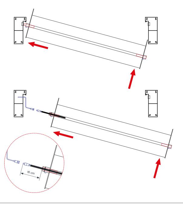
To install the slats, they must be tilted with the end caps facing down, inserting the fixed axle first (left) and then the mobile one (right).
