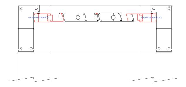
Check that all the "U" profile holes match the M6 machined ones on the beam. If all of them match, apply the sealant between the "U" profile and the beam after screwing the profiles with the USL (ISO 7380) A2x16 screws.
