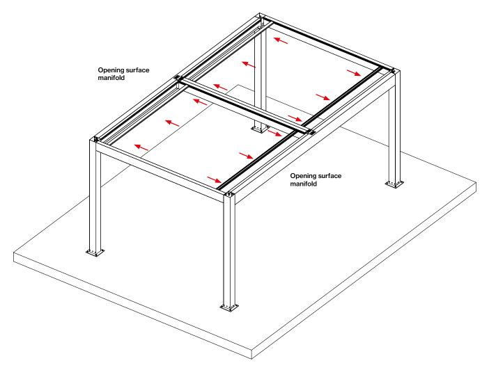
Apply the provided sealant between the contact sides of the opening and closing beams and their corresponding surface manifolds.
