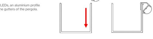
Fit the perimeter LED corner piece shown in the picture on the right to the **corners of the pergola with a column**.
