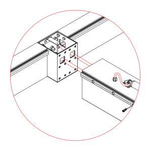
Attaching the central  ${\bf beam}$  to the opening and closing beams. .
