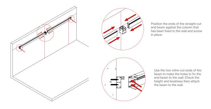
Check that the end beam is level with the base and at the correct height. Check that all marks are at 90° to the base brackets.
