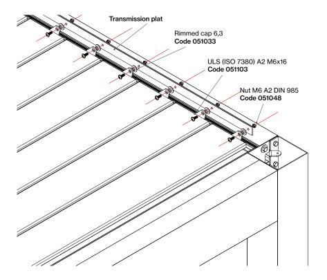
Join the plates to the end caps with their corresponding ULS (ISO 7380) A2 M6x16 screws, 6,3 mm rimmed plastic caps and M6 DIN 985 nut.
