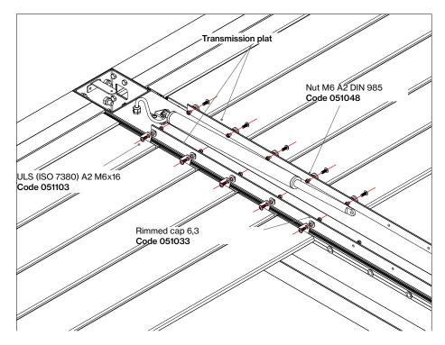
If you prefer, the left and right beam plates can be mounted after all the slats have been inserted.
