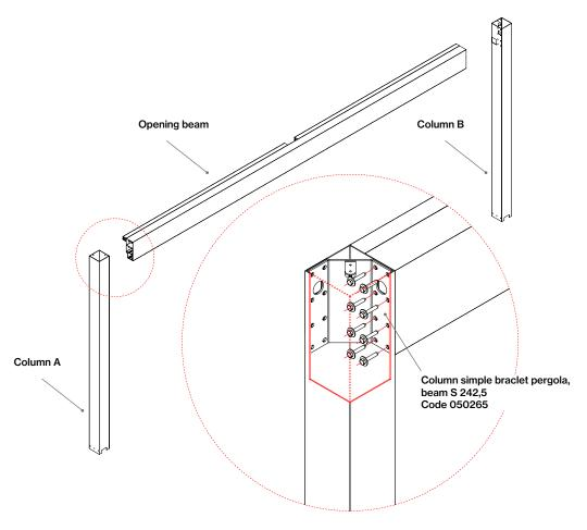
Keeping the opening and closing beams together with the columns, fasten them to the columns bases on the floor surface using the ULS (ISO 7380) A2 M6x16 mm screws. Proceed as shown in the image.
