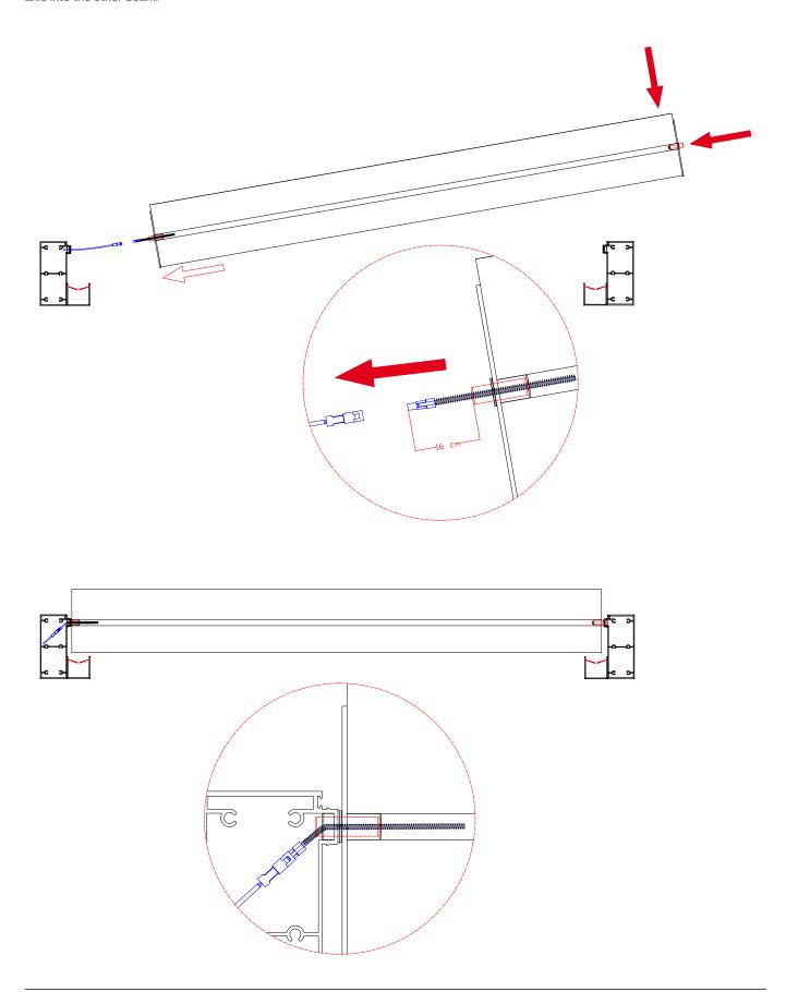
When proceeding to mount the 5th or 6th slat, you will reach the area with the pre-drilled holes in the transmission plates, intended to install the **complete tandem axle set** with code: 050307.
