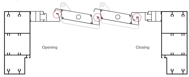
Installing rubber on the clippable opening gutter.
