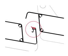
Installing rubber on the slats (150 to 160 slat step).
