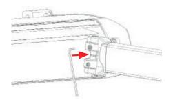
Adjust the height of the elbow so that it closes the box perfectly (if you are using a machine, before adjusting it hold the arms with their cover and release the canvas by operating the machine).
