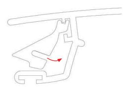
Place the upper register profile in its housing, folding it down until it fits.
