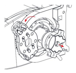
If the motor needs to be dismantled: hold the arms with their cover (first opening the box as necessary) and remove the screws that hold the motor. Remove the screws that hold the motor.
