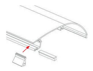
Place the mat profile in the upper register profile (trimming off any excess), then adjust the five wedges so that they are roughly equidistant.
