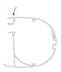
We recommend that you screw the upper register profile to the front, then insert 2 self-tapping ø3.50x13 screws (each approx. 5mm from the end of the profile).
