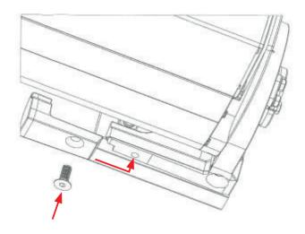
Screw on the two panels that limit movement (vertical and horizontal).
