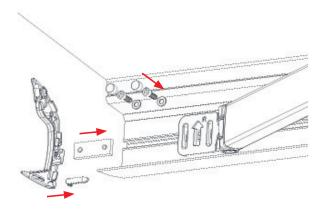
Insert the canvas into the loading bar profile and screw the strips to it. Mount the profile covers. Remove the protective sleeves from the arms.
