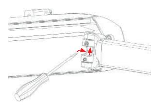
Detail of the extraction of the shaft, in cases where disassembly of the arms is required.
