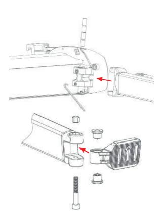
Assemble the invisible Premium arms. Mount the arms in their housing, insert the solid shafts and fix them with the lower pins. Mount the strips to the front terminals.
